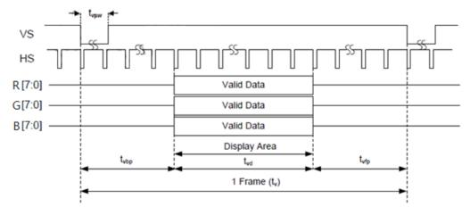
Figure 2 - 12.2. Parallel RGB in SYNC Mode (Vertical)
