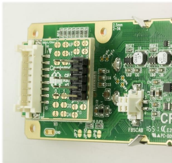
Figure 12. Angled View of CFA-RS232 Level Translator Mounted on CFA735-xxx-KR
