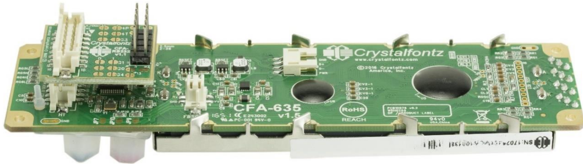
Figure 13. Side View of CFA-RS232 Level Translator Mounted on CFA735-xxx-KR
