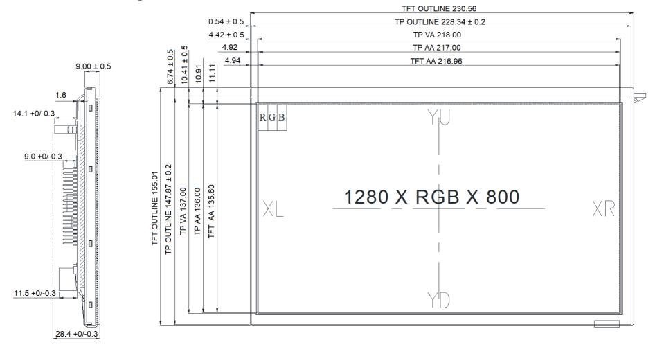
Dimensions are in mm Unless specified, tolerances are ±.3mm
