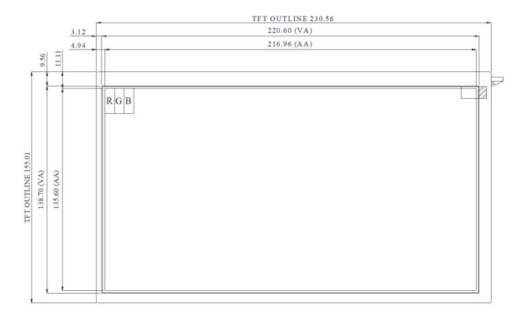
Dimensions are in mm Unless specified, tolerances are ±.3mm
