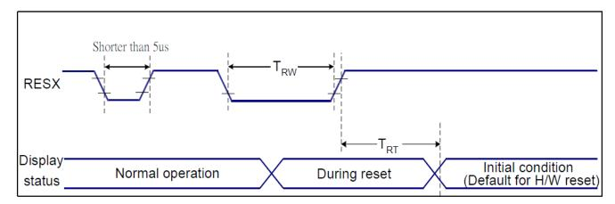
Figure 7 Reset Timing
